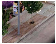
In-ground Planter with Paving Installed: In this image, the pervious paving has been installed above the pavement suspension system. The usable sidewalk area has increased significantly.
