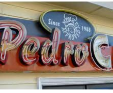
A wall sign utilizing neon tubes; these tubes should be shielded to contain light spill-over.
