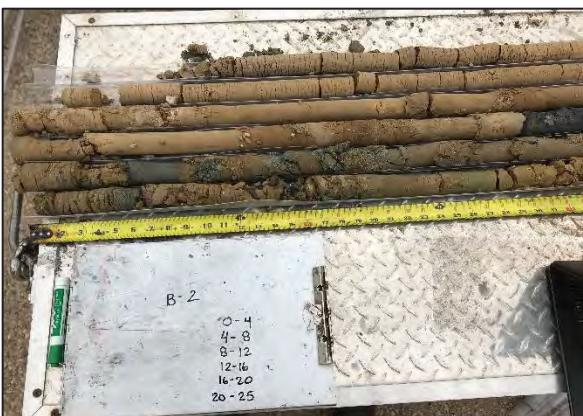
**Photo 5:** Boring 2 was cored from the middle plume area.
